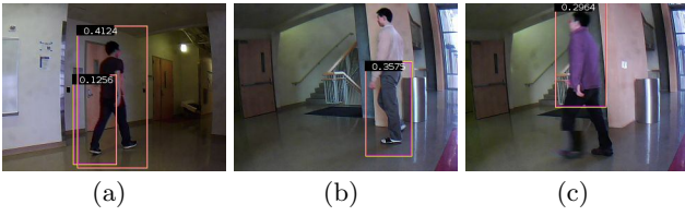
Figure 4: Some false positives from our HOG-based detector. Most of the false positives can be removed using prior spatial knowledge. (a) One bounding box is embedded in the other. (b) The y -coordinate of the bounding box is too large (i.e., the detected person is too small). (c) The y -coordinate of the bounding box is too small (i.e., the detected person is not on the floor).
