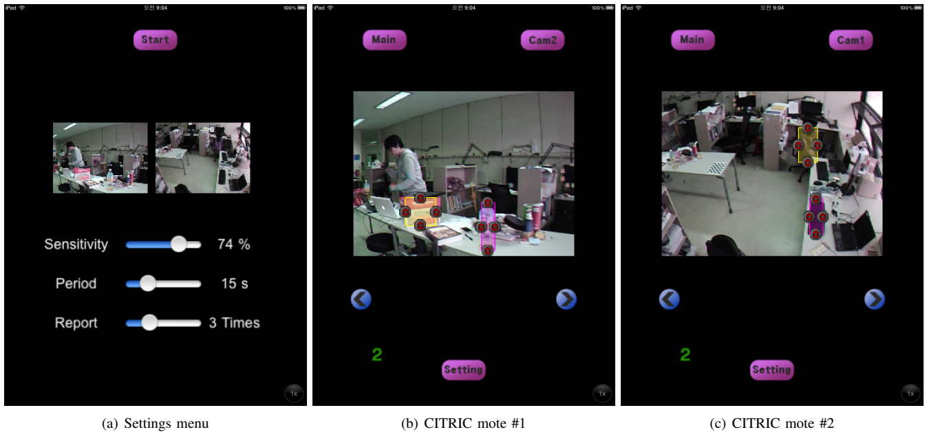
Fig. 4. (a) shows the main settings menu with sensitivity, period and report times. (b) and (c) show how to select the regions of interest. (captured on an iPad for larger screenshots.)
