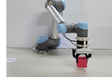
Figure 5: Block placing using a UR-5 robot.
