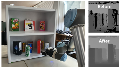
Fig. 6: (left) Real shelf environment with UR5. (right) Post-processing of depth images from the D435 depth camera.
