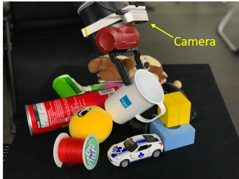
Fig. 1: The grasp detection method proposed in this paper enables 6-DoF grasping by selecting the best approaching direction for 4-DoF grasping. The proposed method especially yields high grasp success rates for a dense clutter of objects as shown in this figure.
