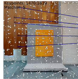
Fig. 2: Target observations (left) and initial observations (right) of failure cases. The keypoints and the matching between the two sets of keypoints are depicted on the figure. The number of keypoints and matchings are written in the text overlaid on the left figures. (a) Insufficient features. (b) Leafage.
