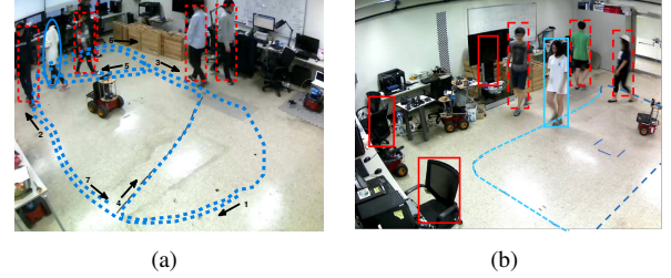
Fig. 5. Experimental setup. (a) The trajectory of a target is shown in a blue dashed line. Other pedestrians (red dashed boxes) generate false detection. (b) A TV, chairs, and sitting persons in red boxes generate static false detections.
