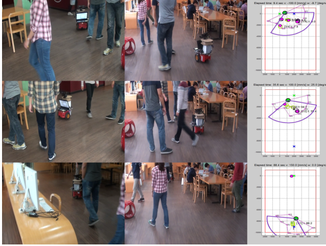
Fig. 6. Snapshots from a real experiment in a crowded school cafeteria. A pink circle represents a prediction of a pedestrian given the observed positions. Each experiment consists of photos taken by camera and robot's internal state. Best viewed in color.
